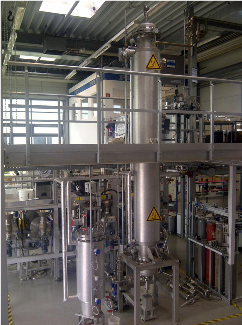
Figure 1: Trickle flow reactor for biogenic methane production in the PFI engineering lab
