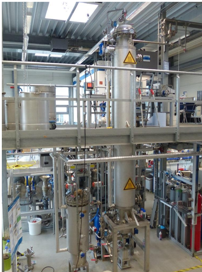
Fig. 1: 300-litre packed bed reactor for engineering lab scale enzyme production
