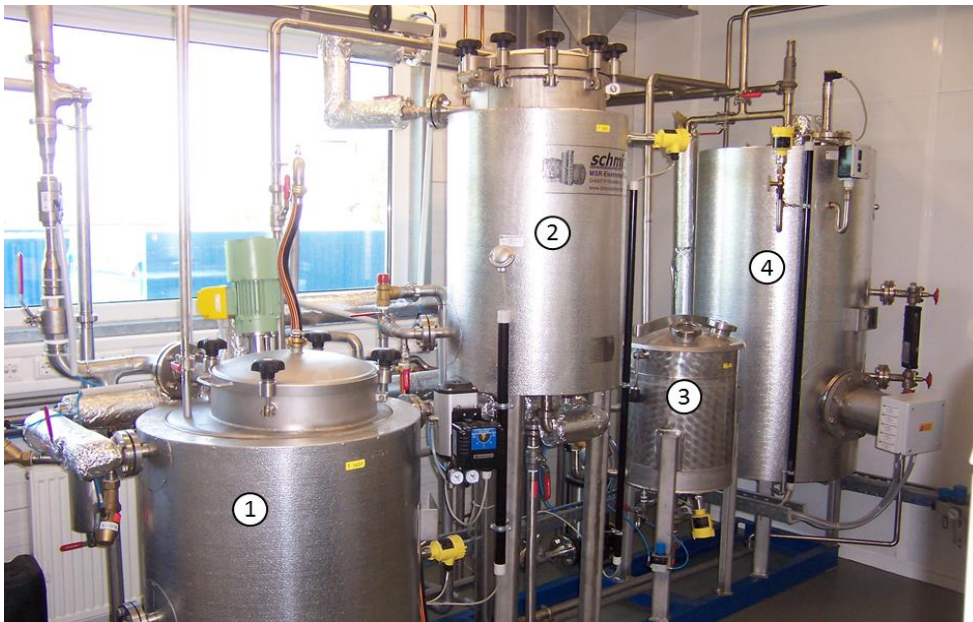
Fig. 3: Pilot extraction unit in the PFI engineering laboratory. 1 = feed tank; 2 = extraction reactor; 3 = receiver; 4 = steam generator
