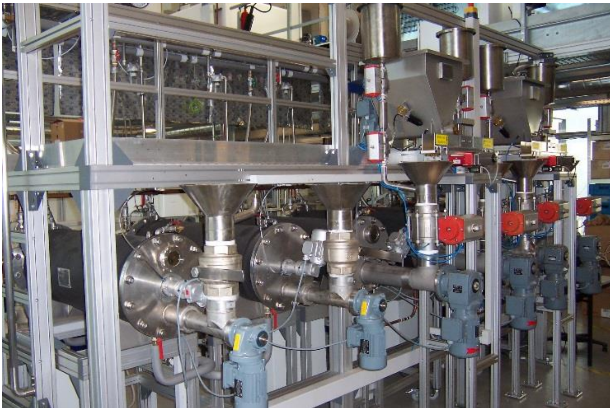
Fig. 1: Static fermentation test (above) and automated continuous fermenter on a 100-litre scale (below) in the PFI engineering lab
